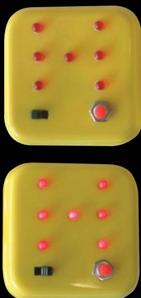
The finished Electronic Dice. The circuit board and battery are encased in a vacuum formed box.
