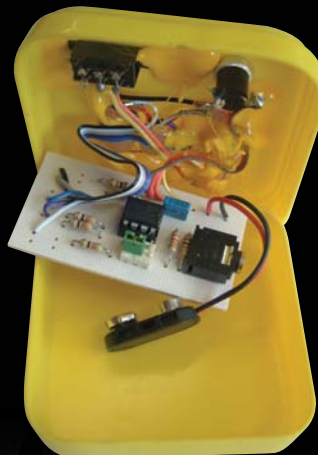
The finished Electronic Dice. The circuit board and battery are encased in a vacuum formed box.
